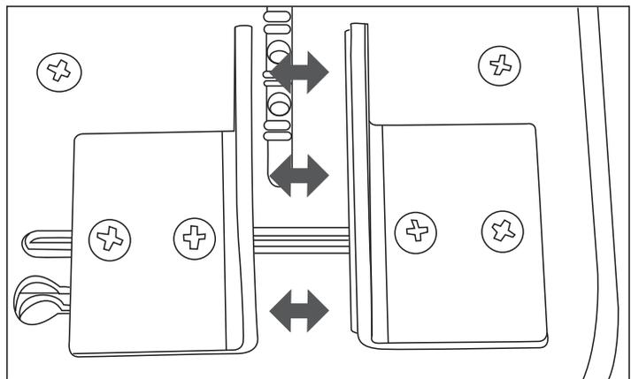
5. Place the thumbscrew into the clamp opposite the one with the foam pad.
