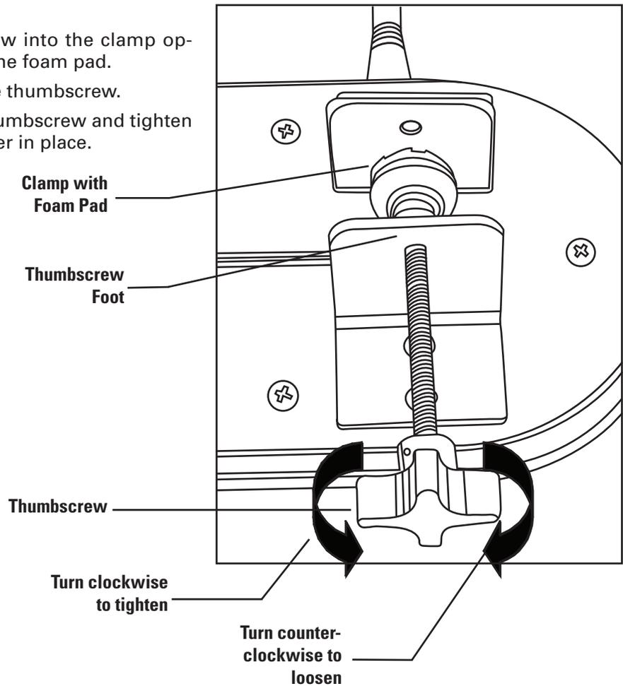
Because the thumbscrews and brackets can be mounted in many ways, they can be adapted to most locations.
